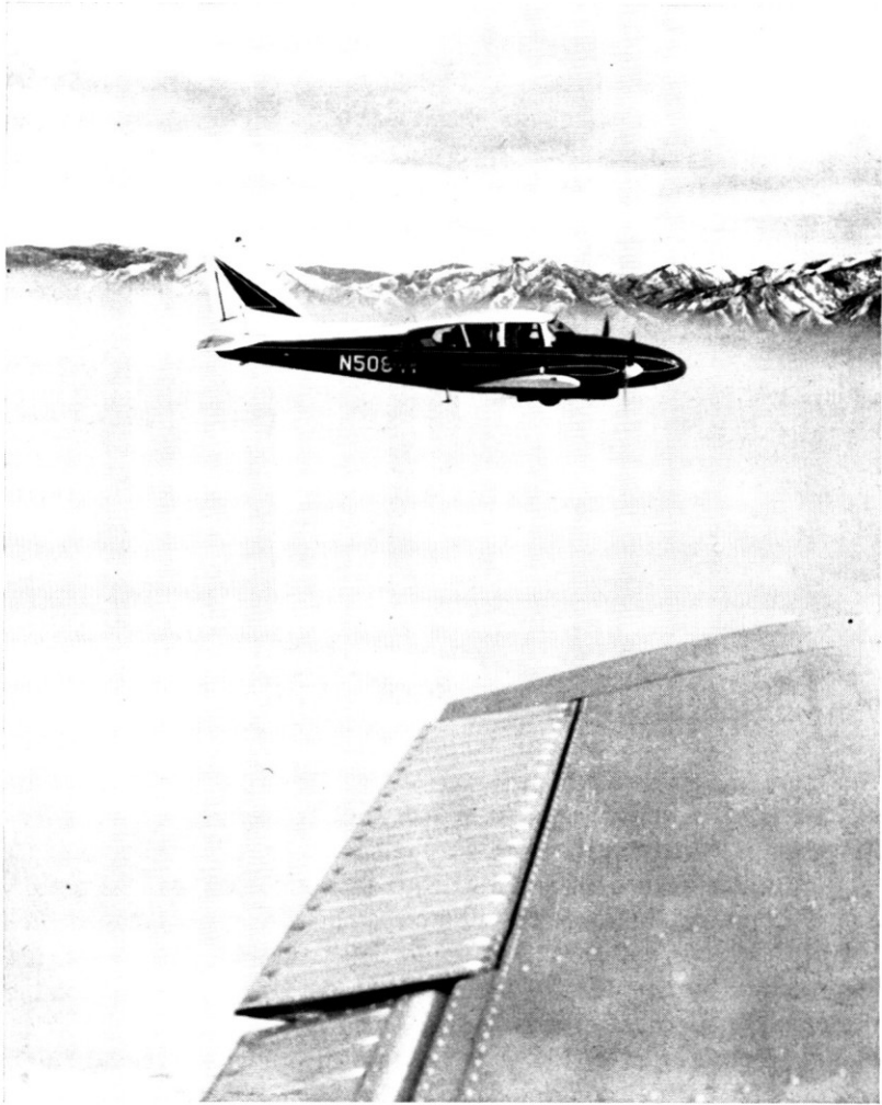
FIG. 2 — Light aircraft employed in dry-ice seeding of supercooled fog in Salt Lake Valley, Utah. Seeding drop is conducted just above top of fog deck
